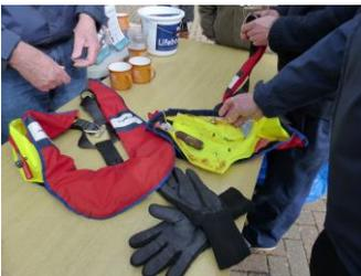
39 jackets were checked at the Lifejacket Clinic. Many had the usual minor faults of no crutch straps, no spray hoods or expired dated accessories, but 3 were condemned as completely useless and one in particular not only had a rusty bottle and rust abraded bladder through the same, but the manual
